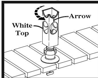
**TURN-** White top 1/4 turn until arrow on side points to slot between boards.
