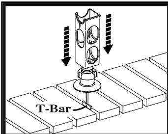
**DROP-** T-Bar all the way through slot between dock boards.
