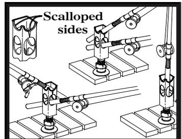
Place rods into holder. Always put rod handle into scalloped sides first. To remove rod, lift up rod and pull out.
