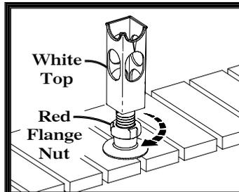
**TIGHTEN-** Red flange nut clockwise while holding white top in place.
